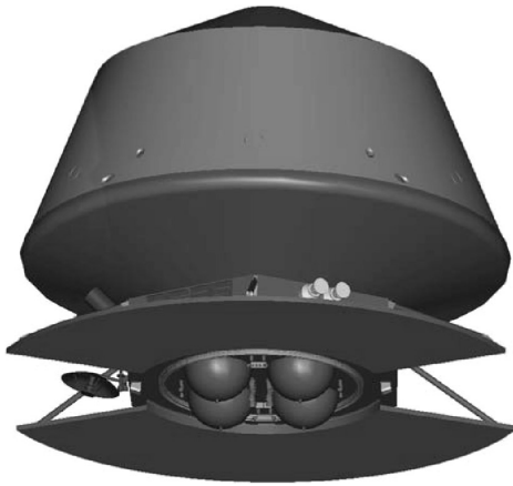
Fig. 2 Mars Science Laboratory entry vehicle and cruise stage (2007 design).
